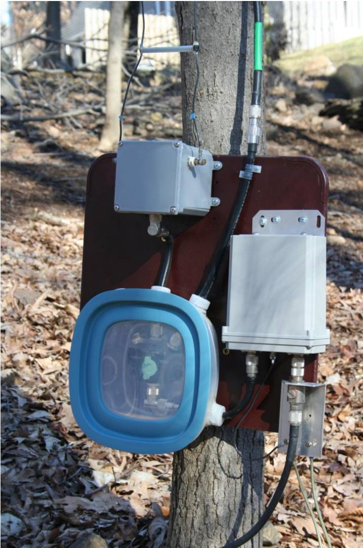
A weatherproof coaxial switch
